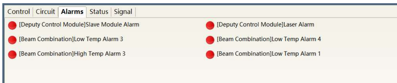
Figure 43 Laser alarm type display area interface
