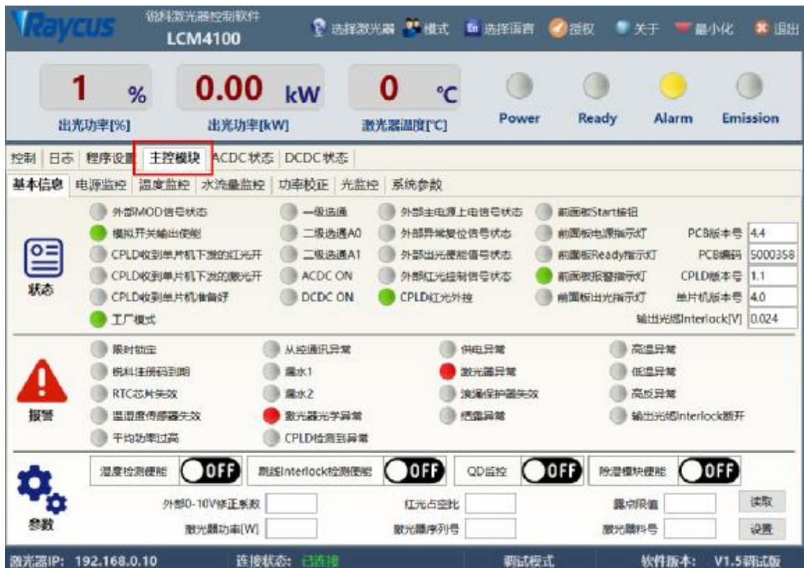
Figure 16 Main control module status information interface
