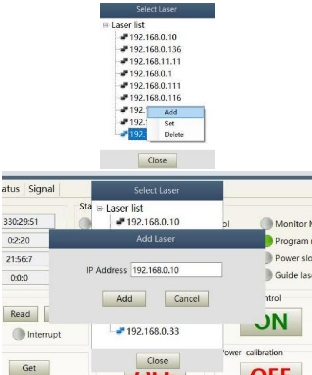
Figure 30 Procedure for adding a laser to the PC software
