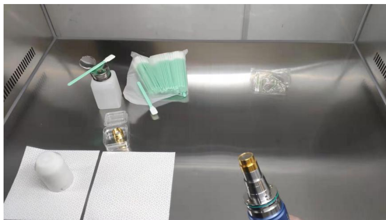
Figure 8 Output optical cable with white dust cover removed
