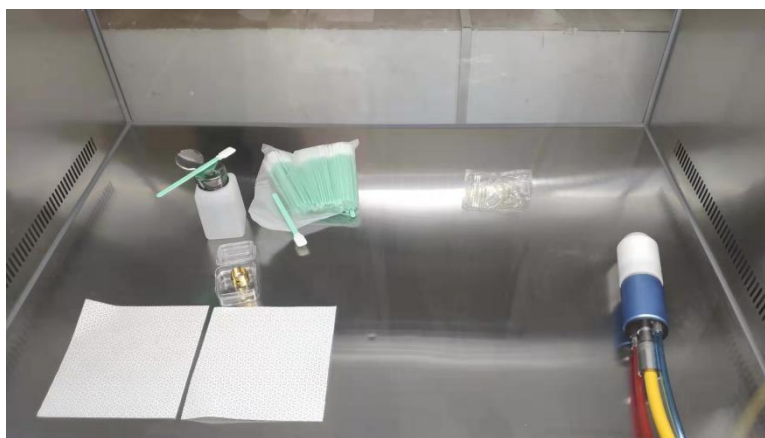
Figure 7 The output optical cable placed in the clean bench with the ventilation turned on
