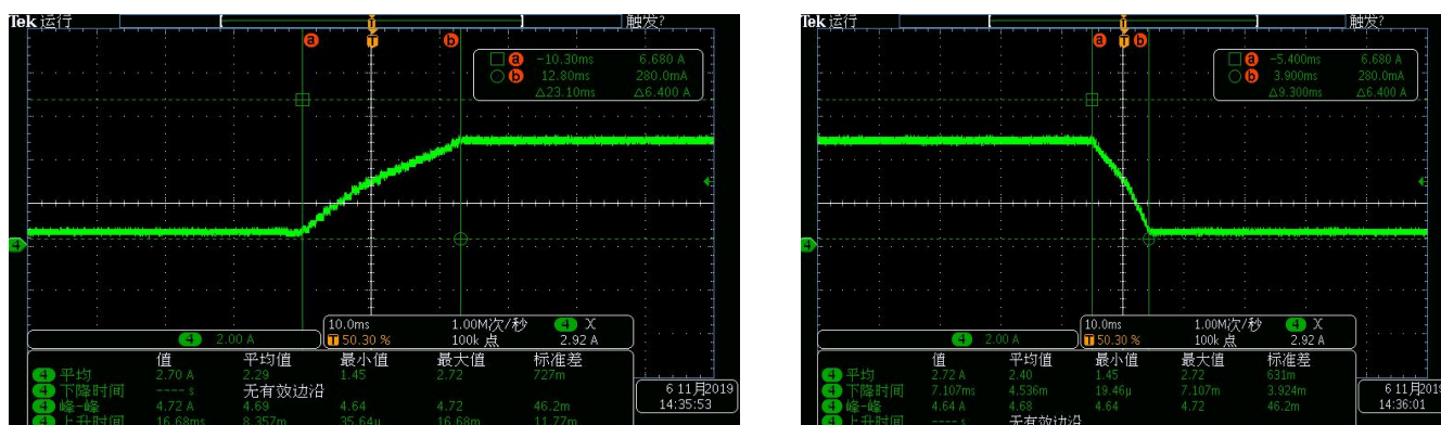
Figure 37 The power slow rise and fall setting area interface and measured programmings
