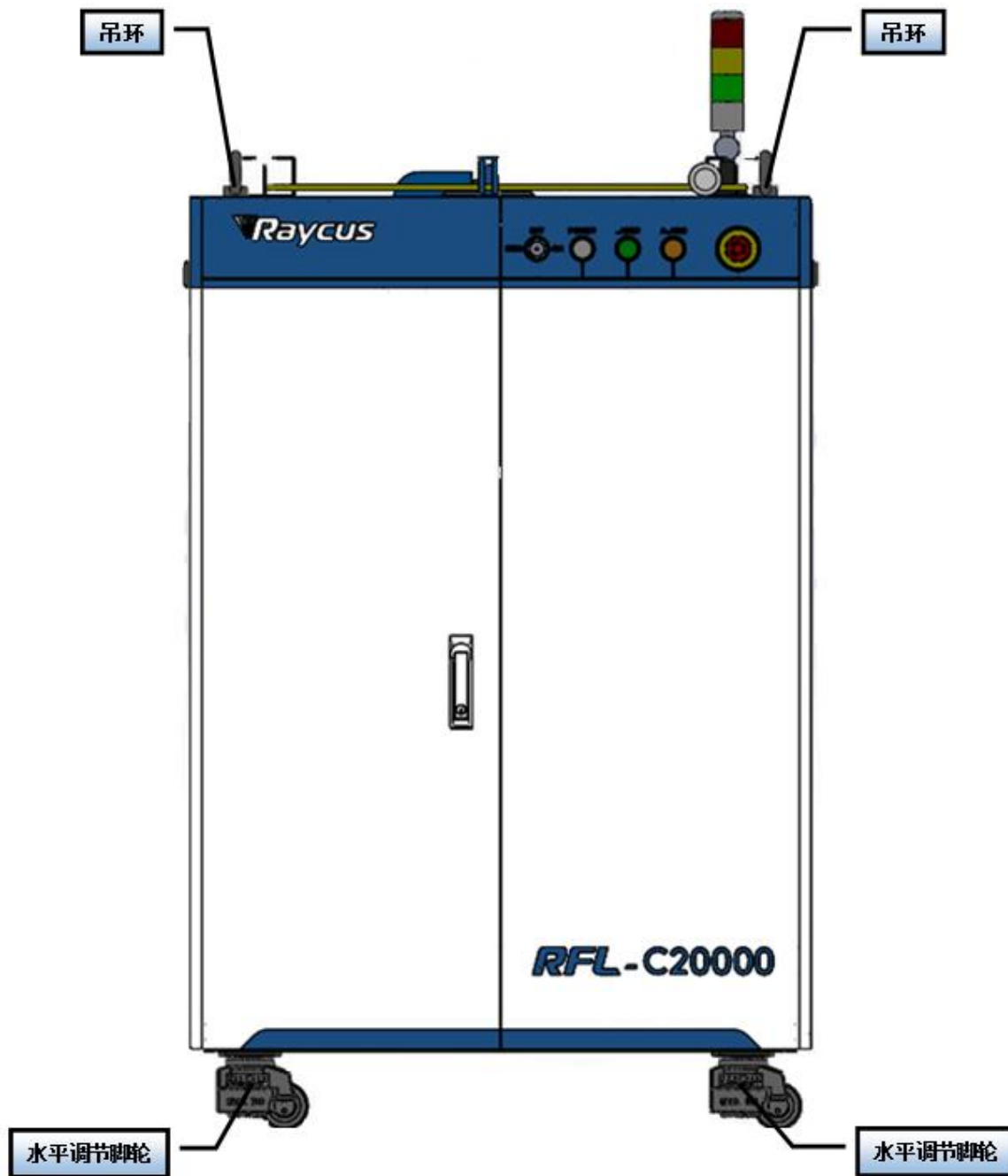
Figure 4 Laser top lifting ring and bottom level adjustment caster.
