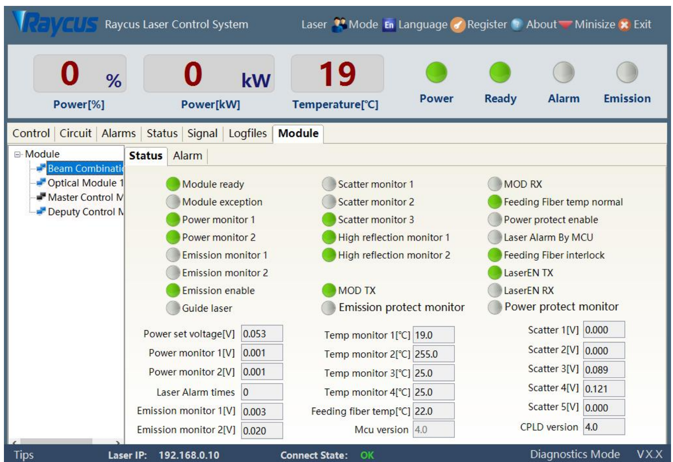
Figure 45 Module parameters query interface in diagnostic mode
