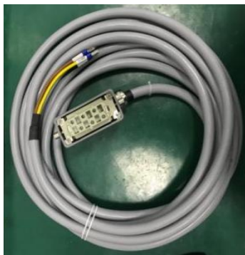
(a) Power cord of 4kW laser
