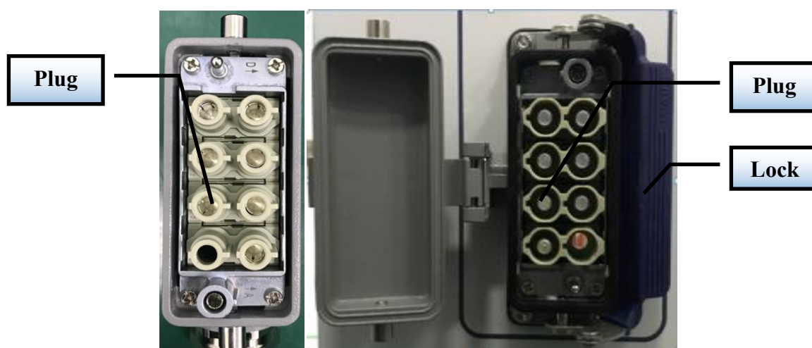
(c) Power cord plug and socket of 8kW/10kW/12kW laser
