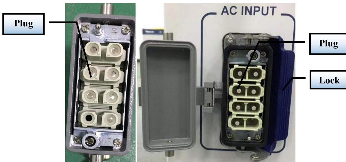
(b) Power cord plug and socket of 6kW laser
