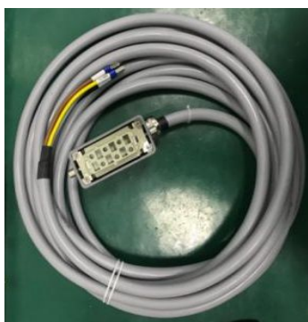
(a) Power cord of 4kW laser
