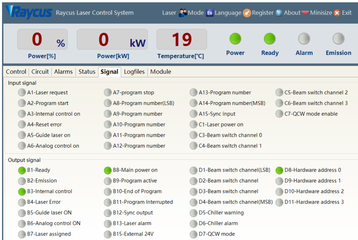
Figure 46 The interface status in diagnostic mode
